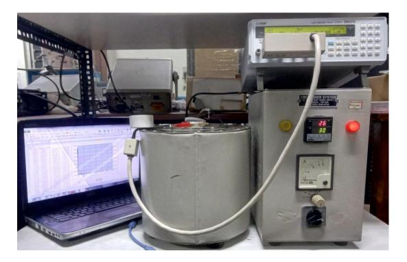
Fig. 2.17: Dielectric properties measurement setup.
