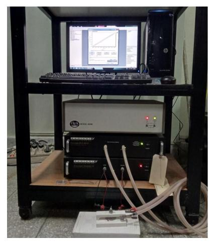
Fig. 2.20: The Polarization vs Electric Field hysteresis loop measurement setup.
